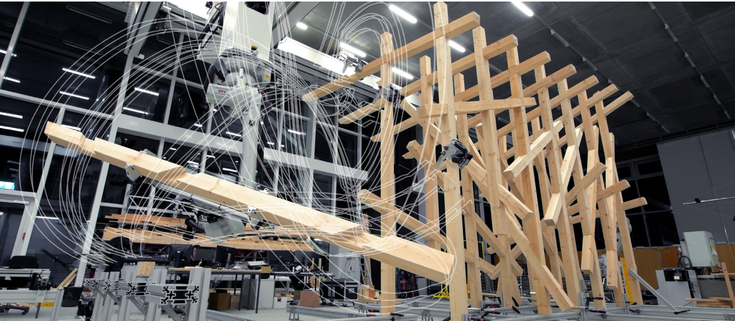
1 Robotic Motion trajectory created for timber assembly process (Pok Yin Victor Leung, 2021, © Gramazio Kohler Research).
