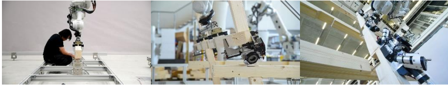
Fig. 4. Photos showing a snapshot of the three assembly methods: Ground Connection (left), Joint Clamping (middle), and Joint Screwing (right)
