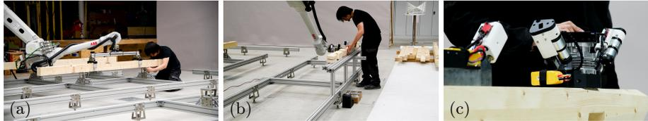
**Fig. 3.** Image showing the manual actions (a) fixing ground elements to the platform, (b) loading timber element onto the gripper, and (c) attaching screwdriver onto the timber element.
