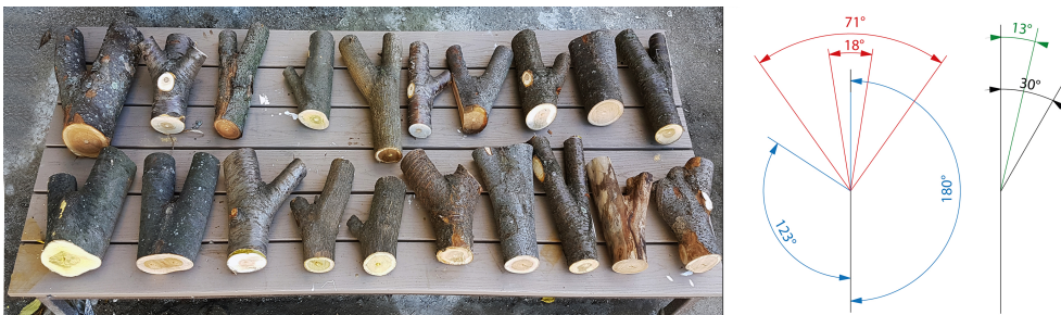
Figure 4: Collection of Y-shaped branches and their combined geometric range (top view and side view)
