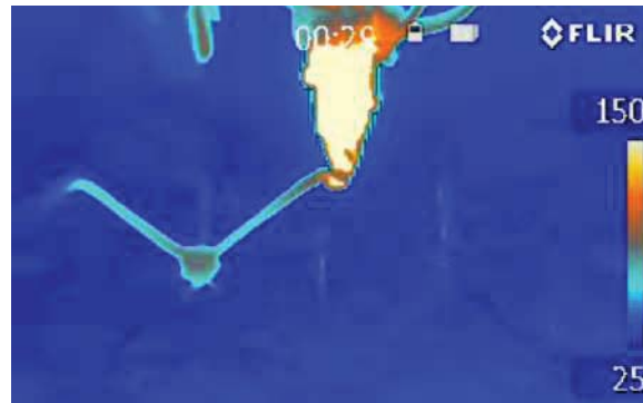
Figure 23 Temperature profile of the end of a recently extruded member as the printing of the subsequent member commences (see online version for colours)
