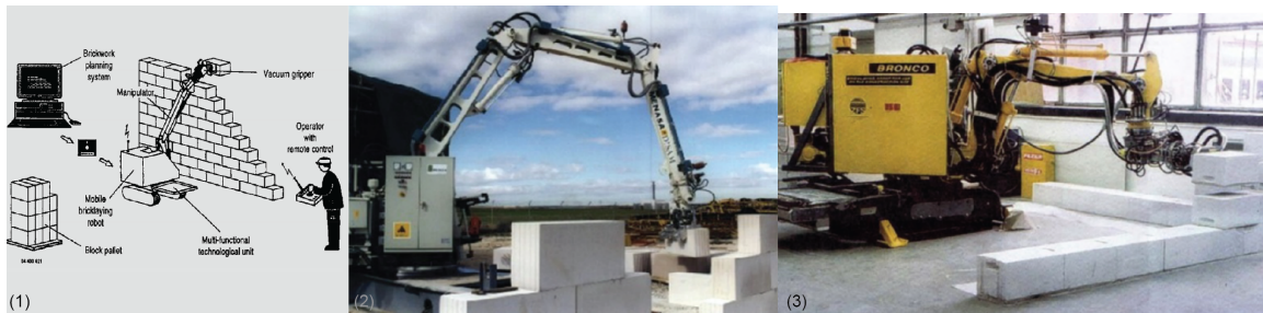
Figure 2-10: (1-2): the EU Robotic Assembly System for Computer Integrated Construction (ROCCO) [GBG00]; (3) the Bricklaying Robot for Use on the Construction Site (BRONCO) [PDKG96]. Images by corresponding papers.
