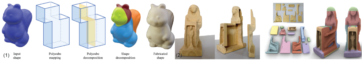
Figure 2-25: Examples of height-field decomposition methods:(1) Two-step approach based on polycube mapping [FCM+18]; (2) Optimization-based approach [MLS+18]. Images by corresponding papers.
