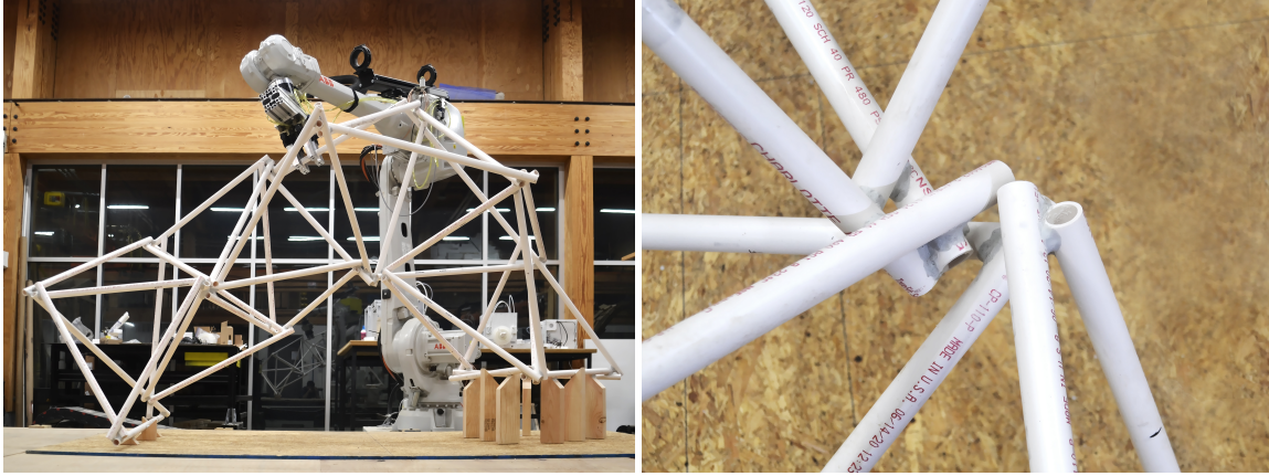
Figure 4-6: Short Arch; left : the completed structure; right : a detailed view of a joint.
