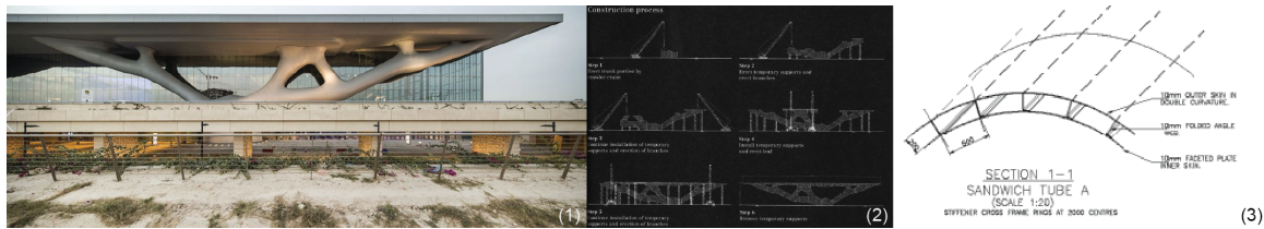
Figure 2-5: The design of the Qatar National Center’s facade. (1) picture of the finished structure, photo credit to Nelson Garrido; (2-3) the detailed construction sequence and the sandwiched skin conceived originally by Matsuro Sasaki, image from [MS08].
